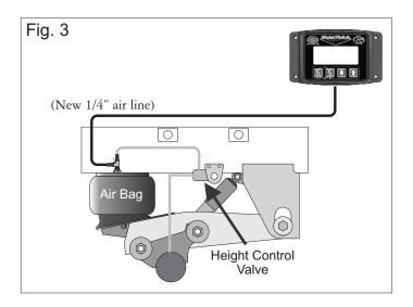
Step 7: Air-up the suspension system and check all fitting connections for air leaks.
