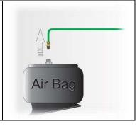
Insert the Street Tee fitting into the top of the air spring and then reattach the suspension airline into the Street Tee.
