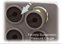
c) Cut a new hole in the dash panel using a 2-1/16 inch (52 mm) hole saw.
